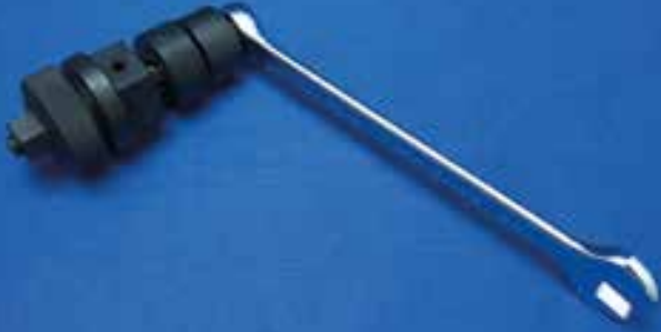
Figure 6 - Disassemble tool using spanner
